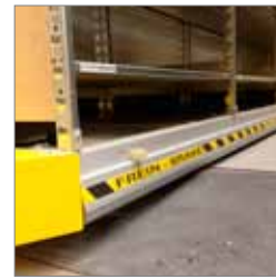
Mechanical Safety Brake
